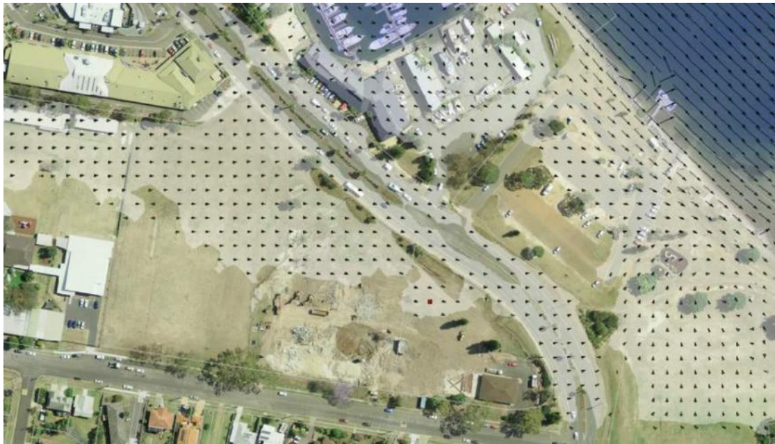
Figure 24: 1:100 yr flood level, depth and velocity as advised by PMHC in 2018
